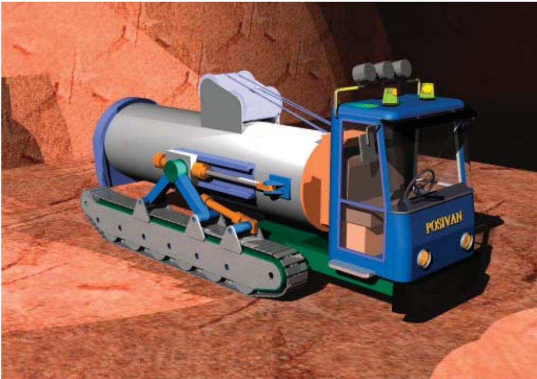
*Assuring the fire safety is one of the bases for design of the canister transport vehicle.*
