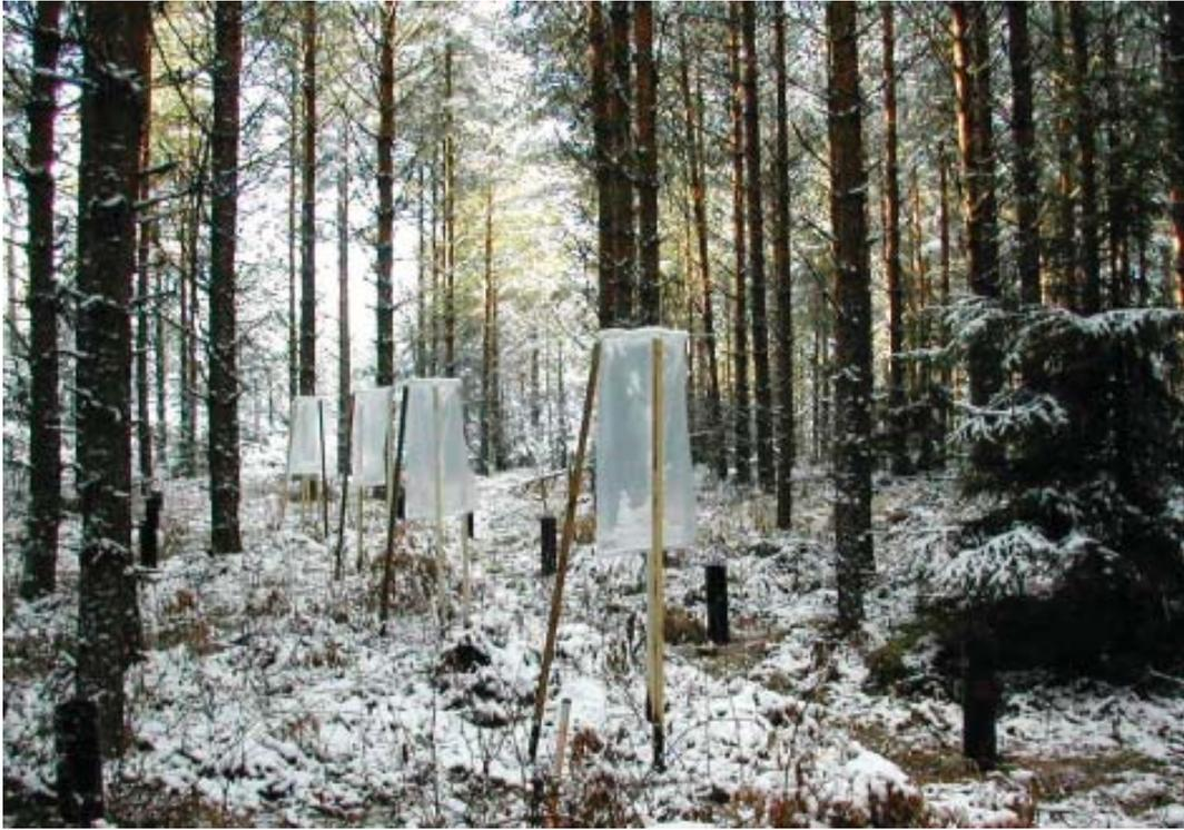
*Snow collectors erected in an intensive observation area inside a forest stand, which help examine, for instance, the effects of treetops on the chemical composition of falling rain and snow.*
