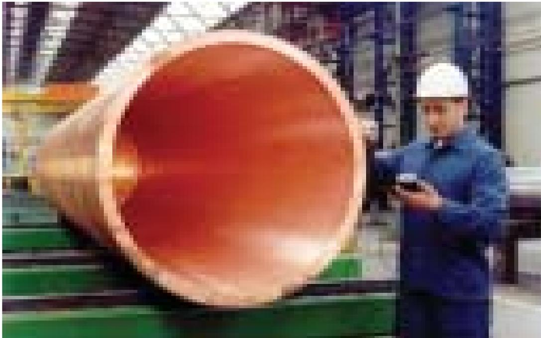
*The first canister casing fitted with an integrated bottom manufactured at the factory of Vallourec & Mannesmann Tubes after pre machining.*
