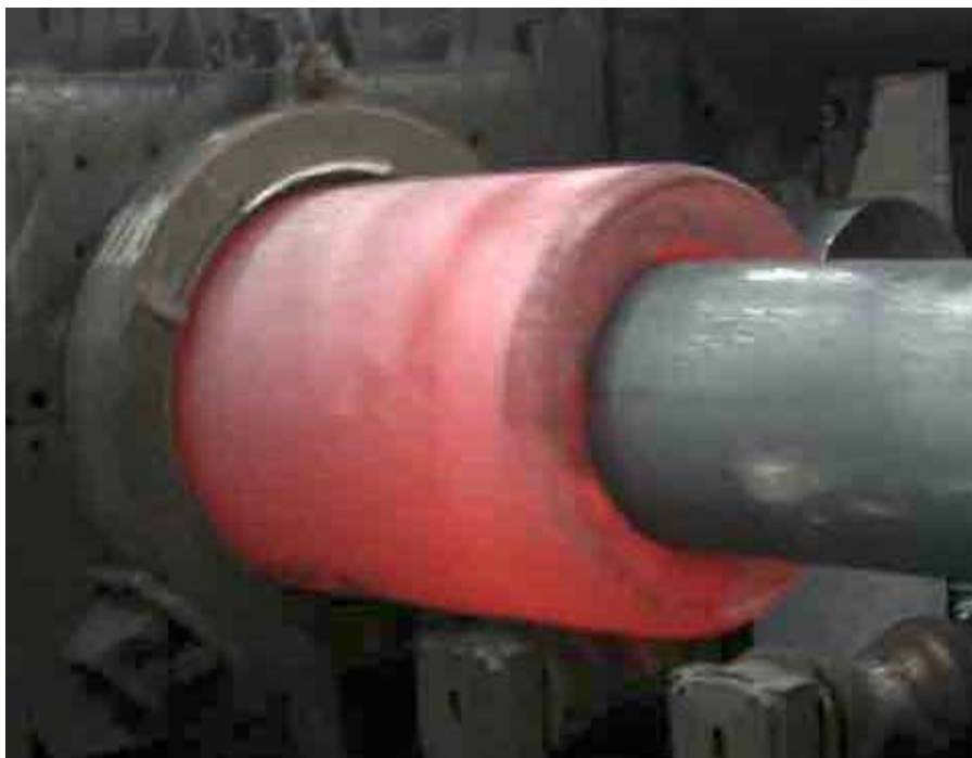
Draw of the canister being done at the pipe factory of Vallourec & Mannesmann Tubes in Germany.
