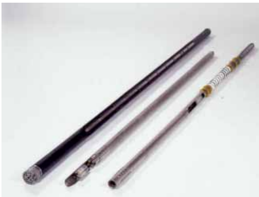
Development projects of the flow measurement equipment were underway mainly to improve electronics of the differential flow measurement units and to widen their measuring range, particularly to enable the measurement of ever-smaller flows. The figure shows the borehole transducers that are being used in the flow measurement units.
