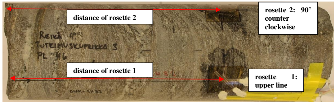
Figure 3-1. Illustration of rosettes' positions. Distance was measured from the bottom of the sample to the centre of the rosette.
