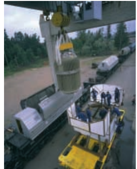
For 16 years, fuel was returned from Finland to the Soviet Union. Transfer of a transport cask from vehicle to train wagon. The locomotive speed limit was 40 km / hour.
