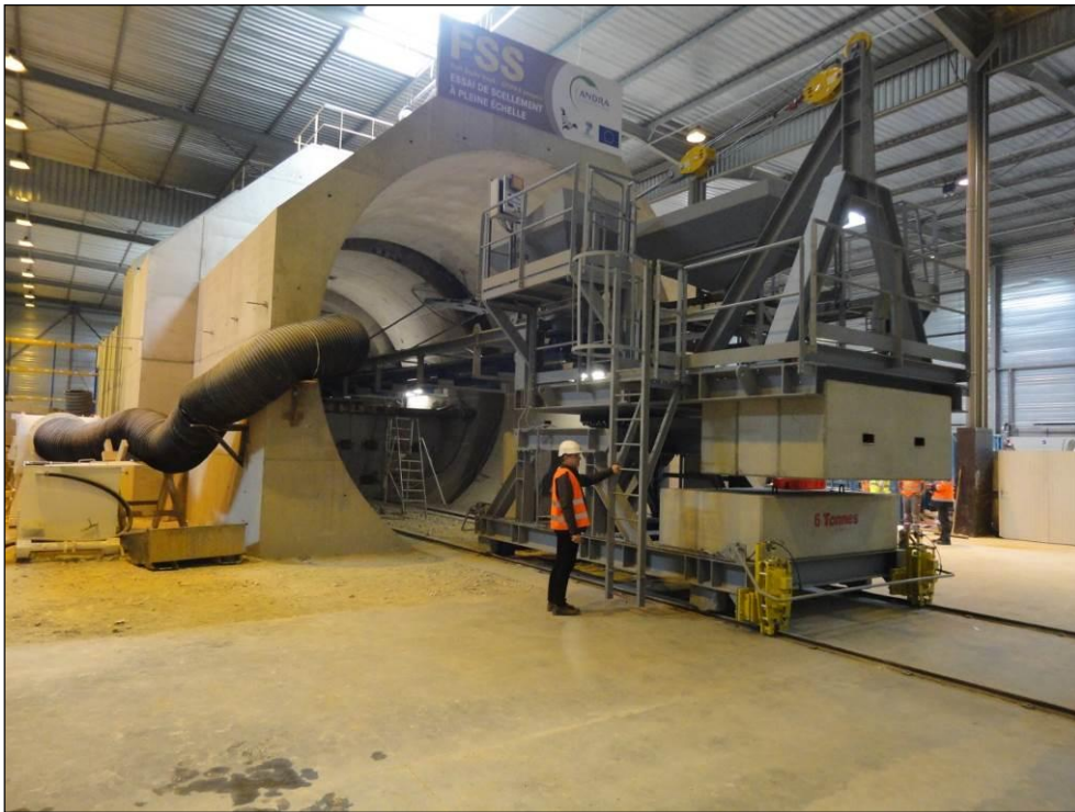
Figure 2.13: The bentonite emplacement machine.
