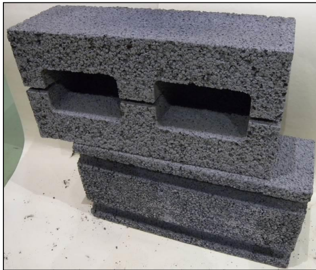
Figure 5.5: Low-pH LECA ® blocks used for the filter layer in the POPLU experiment.
