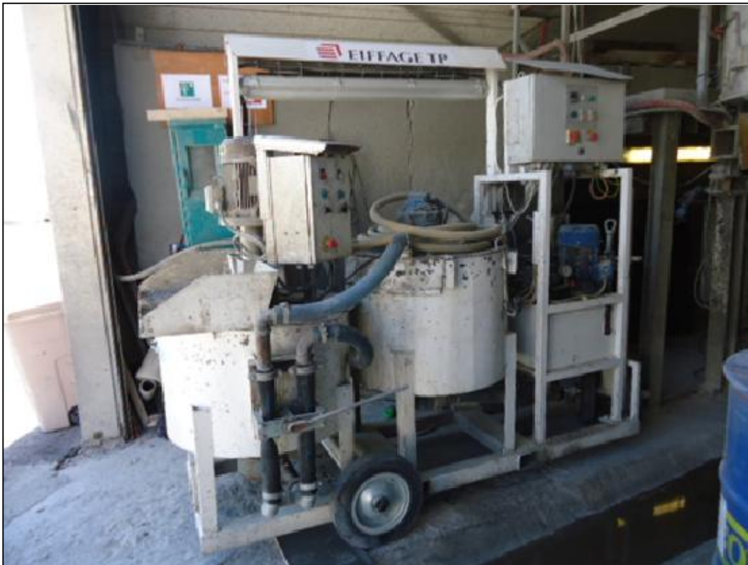
Figure 2.12: Grouting machine used in the FSS experiment.
