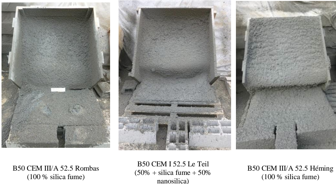
Figure 2.6: Photographs of the outcomes from the test spraying of metric test panels.
