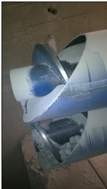
Figure 2.15: Transferring the bentonite into the filling machine using forklift trucks (left) and then transfer of pellets through a conveyor belt into the auger (right).
