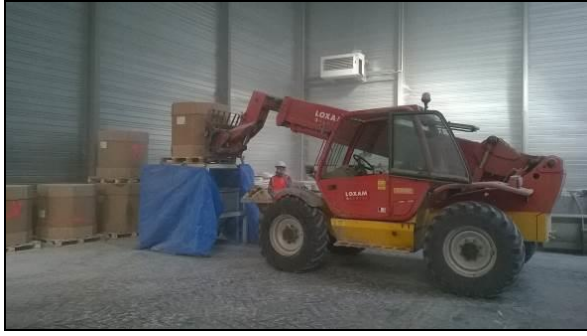
Figure 2.14: Emptying of an octabin containing bentonite pellets (left) and a big bag with bentonite powder (right) into hoppers.
