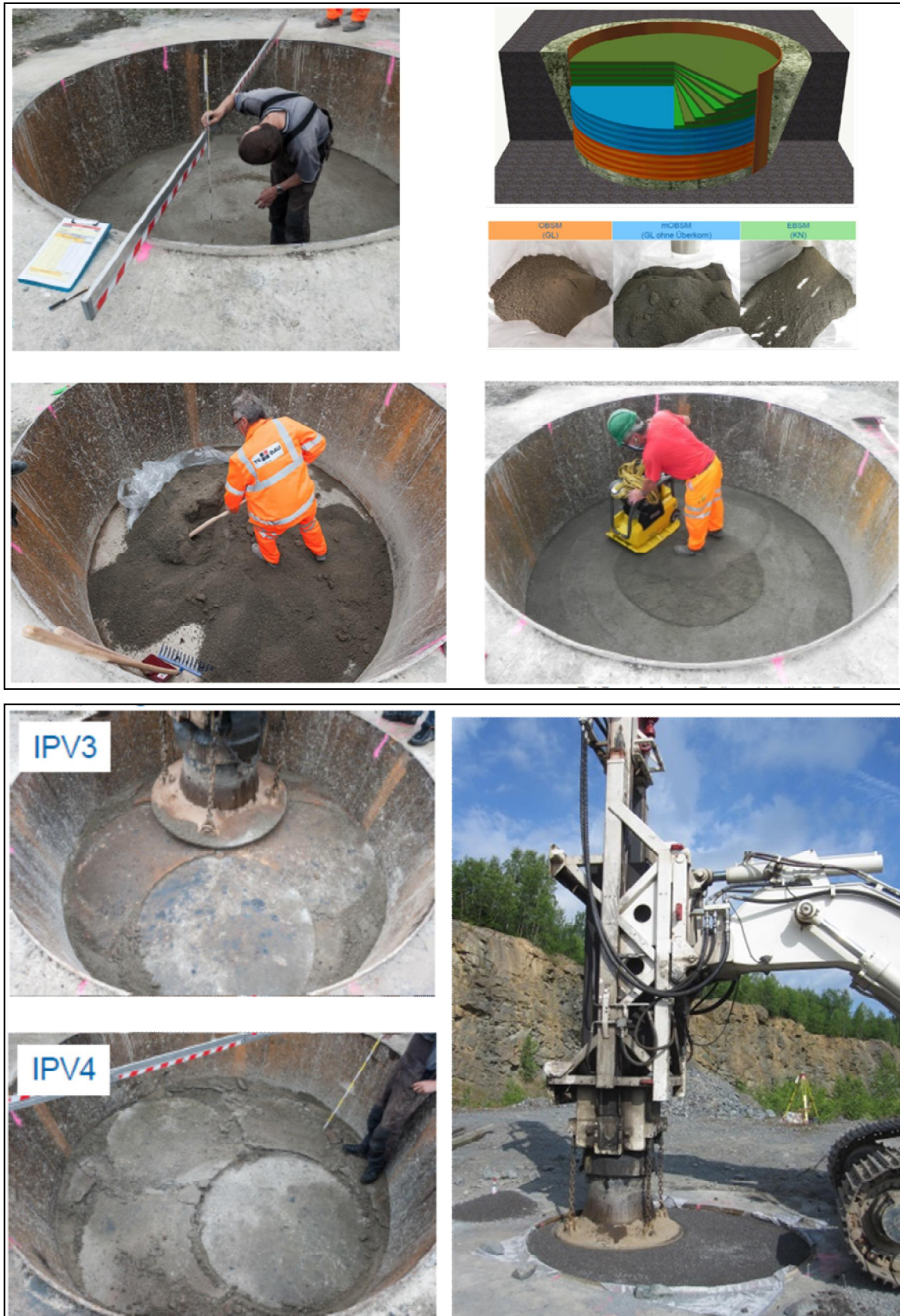
Figure 6.5: In situ compaction test using pre-compaction by vibrating plates and pulse compaction with high impact forces for of crushed salt and clay mixtures - © Uwe Glaubach, TU Bergakademie Freiberg.
