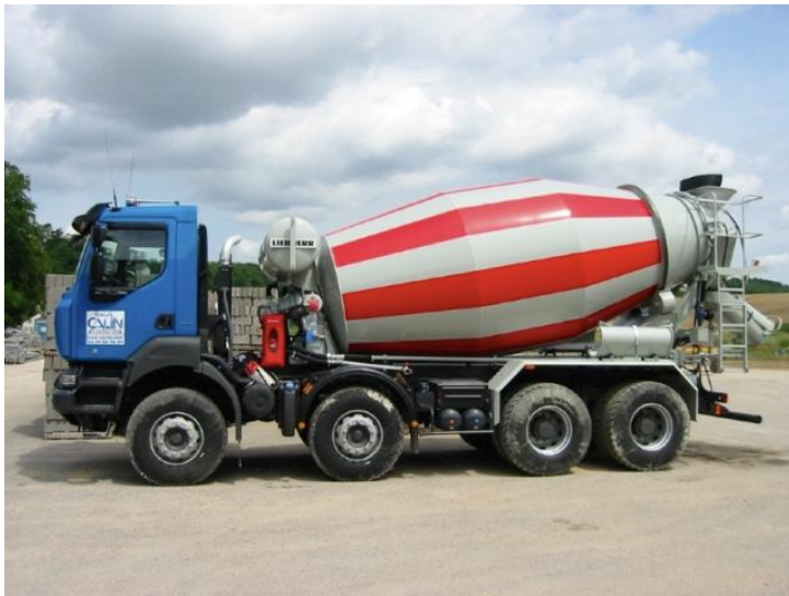
(a) Concrete mixer-truck used to carry concrete © Paul Calin
