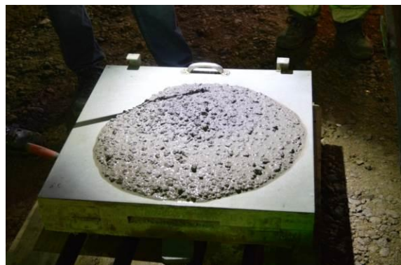
Fresh concrete measurement of slump flow, underground during quality control before pumping.
