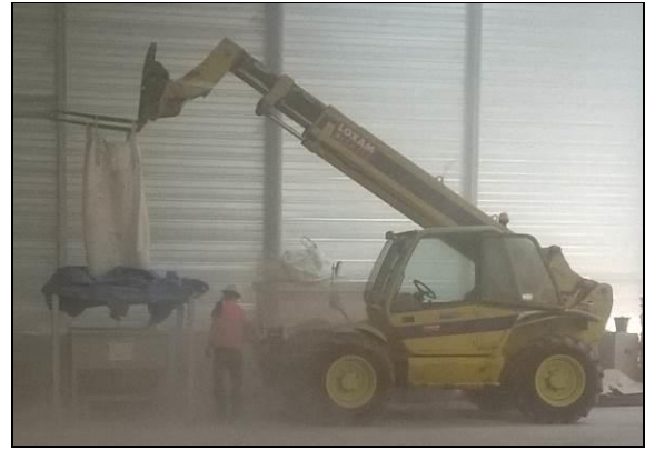
Figure 2.14: Emptying of an octabin containing bentonite pellets (left) and a big bag with bentonite powder (right) into hoppers.
